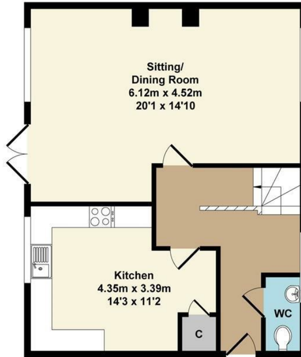
Sitting/ Dining Room 6.12m x 4.52m 20'1 x 14'10 Kitchen 4.35m x 3.39m 14'3 x 11'2 WC Ground Floor Approx. Floor Area 50.60 Sq.M. (545 Sq.Ft.)
